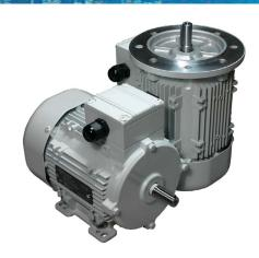
Anaheim Automation's AC Industrial Motors come in two different mounting options: Leg (foot) mount and the flange mount option. Both the ACI-PMEJ075-4R4LAT and the ACI-PMEJ075-4R4FAT run up to 1,710 RPM and deliver 750 Watts of power. All of our ACI-PMEJ075 AC Industrial motors are 3 phase, and can be wired to run off of 220VAC or 380VAC at a frequency of 60Hz.
